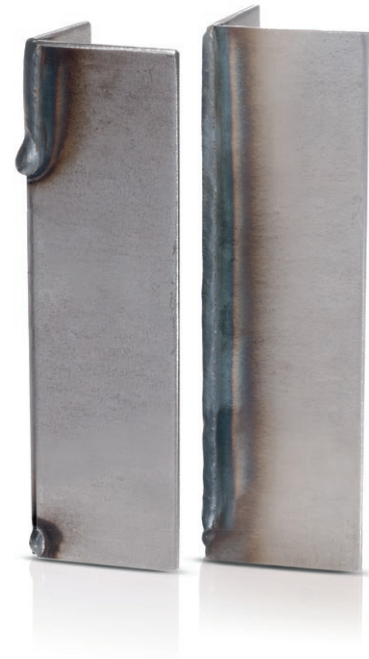
A welded corner seam as a comparison. Standard arc (left): Rapidly falling weld pool that is about to drop off. SpeedCold (right): Welded in full with utmost speed and reliability (35 cm/min).
